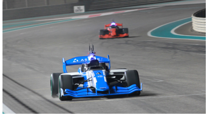
Fig. 1. The EAV24 racing vehicle of TUM Autonomous Motorsport used during the Abu Dhabi Autonomous Racing League. It is based on Dallara’s SF23 Super Formula Chassis and contains an autonomous driving hardware stack in the space usually occupied by the driver.
