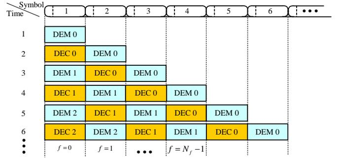
Fig. 2: OFDM-symbol processing procedure in the pipelined IDD
