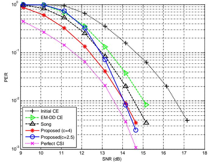
Fig. 9: PERs with different channel estimators:  $2 \times 2$  SM-MIMO-OFDM (7 iterations)
