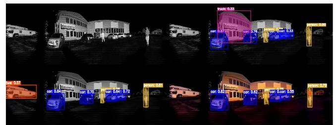
(b) Instance segmentation on lidar reflectivity image
