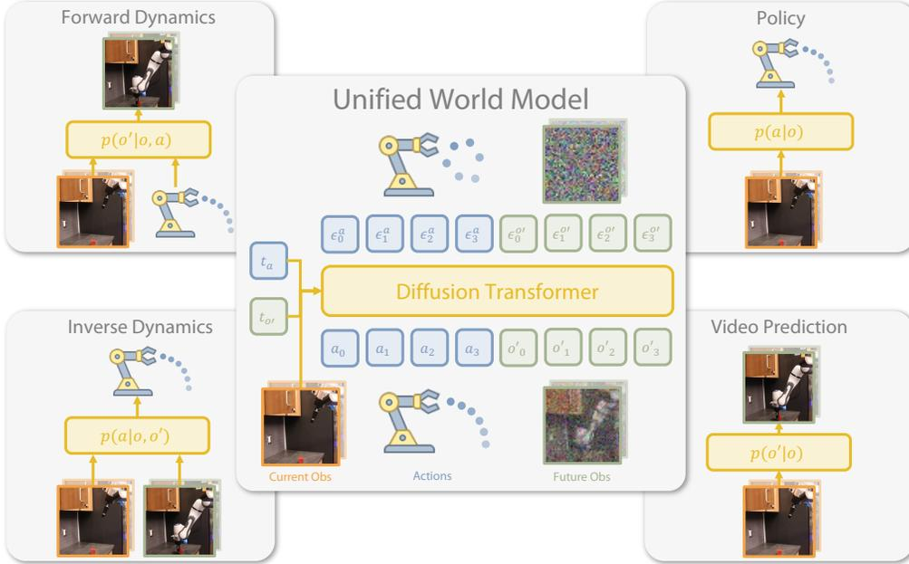
Fig. 1. Unified World Models integrates action and video diffusion in a unified transformer architecture controlled by modality-specific diffusion timesteps. The model can flexibly be trained on large robotics datasets and then flexibly perform a variety of different inferences at test time. Doing so naturally enables improved robustness and generalization for imitation learning.
