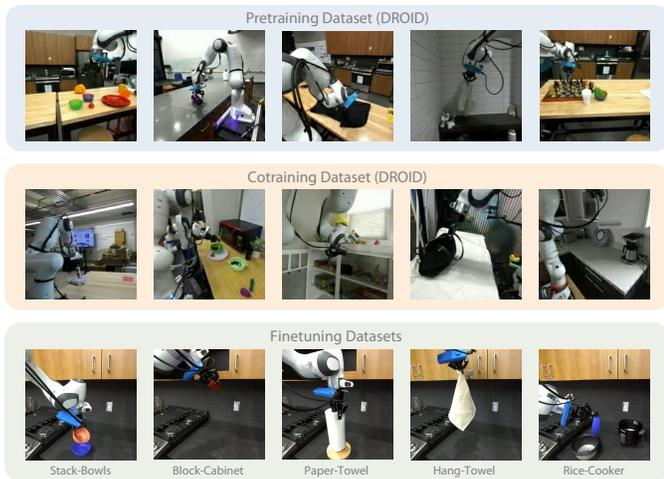
Fig. 4. Visualization of datasets used for pretraining and finetuning. The pretraining/cotraining dataset consists of diverse tasks performed by Franka robots in various environments to ensure broad generalization capabilities. The finetuning datasets include five tasks, each designed to evaluate task-specific performance under controlled conditions.
