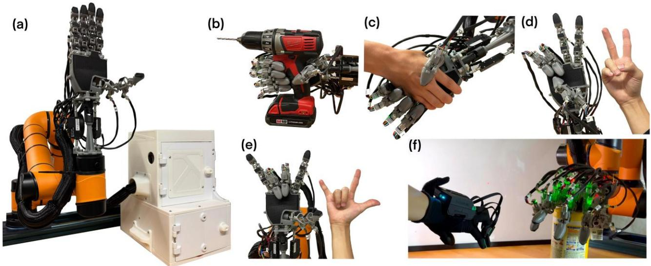
Fig. 1. The developed Krysalis Robotic Hand (a) mounted on a AUBO i5 cobot, with its umbilical cord and the robot control unit (RCU), (b) holding a power drill machine, (c) shaking hand with a human, (d) making victory 'V' sign, (e) making the "I Love You" sign, (f) being teleoperated in real-time.
