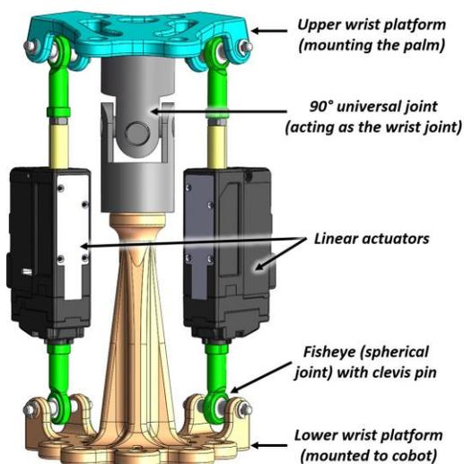
Fig. 7. The mechanism of the wrist module.
