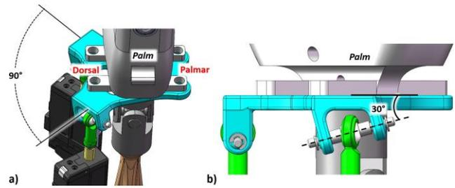
Fig. 8. The design of the upper wrist platform with (a)  $90^\circ$  offset between the two linear actuators and (b)  $30^\circ$  angle between the horizon and the spherical joint axis.
