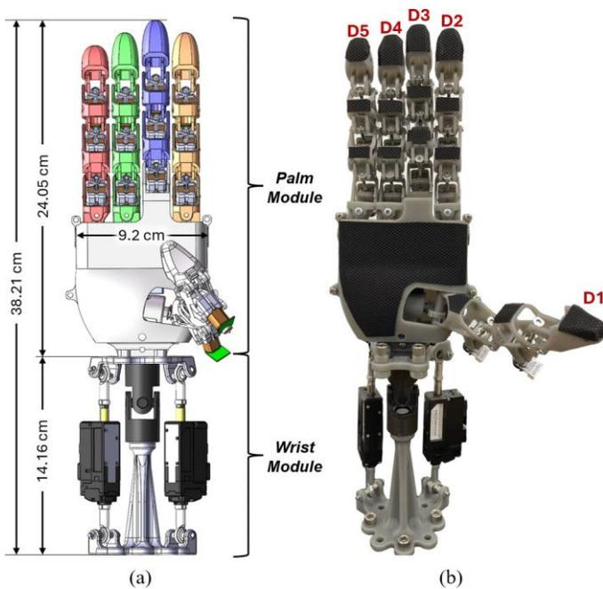
Fig. 2. The Krysalis Hand (a) CAD assembly showing wrist and palm modules, with fingers in different colors (b) designed and implemented robotic hand with finger numbering.
