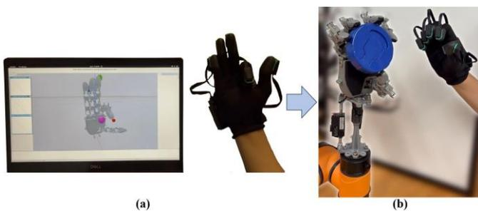
Fig. 15. Teleoperation setup showing real-time (a) URDF control in the PyBullet environment (b), which broadcasts the ROS 2 messages to the Krysalis Hand.
