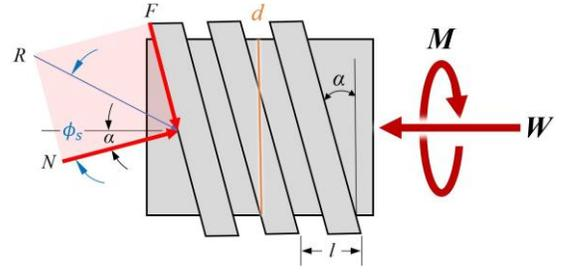
Fig. 4. Free body diagram of the screw.
