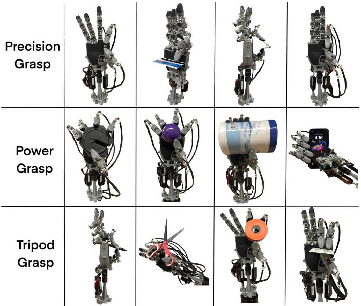
Fig. 14. The grasping capabilities of the Krysalis Hand with various payloads, categorized into precision, power, and tripod grasps.
