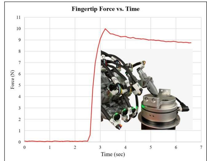
Fig. 10. Active fingertip force as a function of time.
