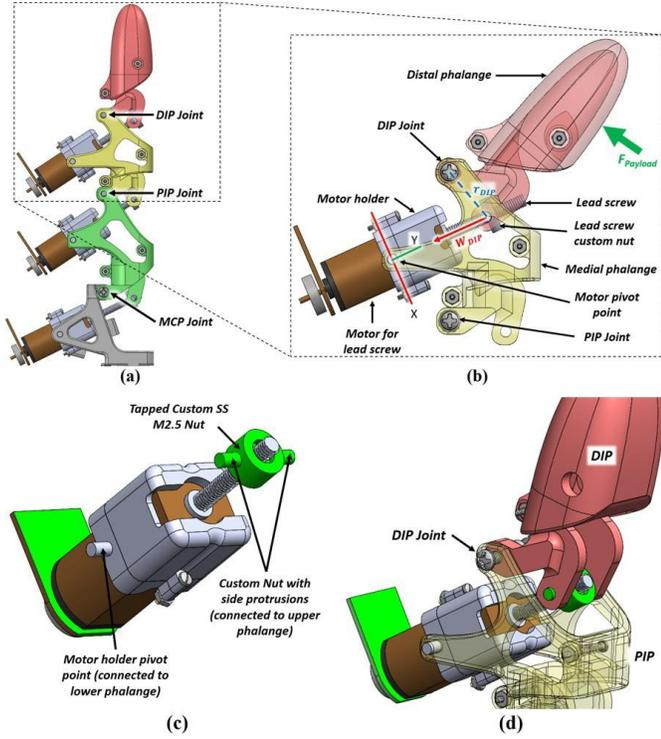
Fig. 3. (a) Entire finger assembly, (b) Leadscrew actuation mechanism in detail, (c) Schematic of motor and custom nut in isolation, (d) Schematic showing the custom nut engaged to the phalange above it (DIP in this case).
