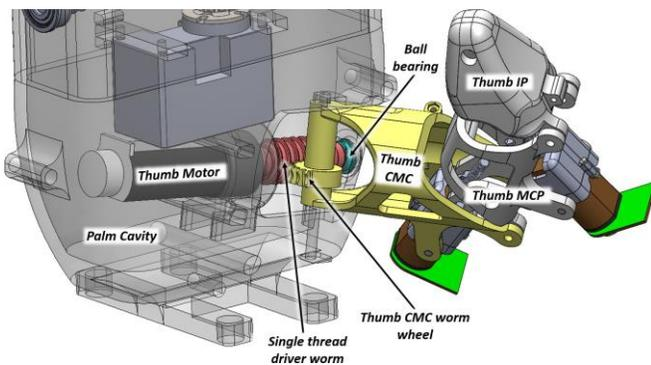
Fig. 5. Thumb CMC joint mechanism.
