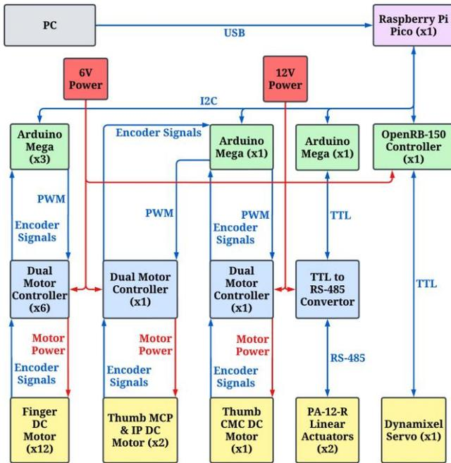
Fig. 9. Electrical block diagram of the Krysalis Hand
