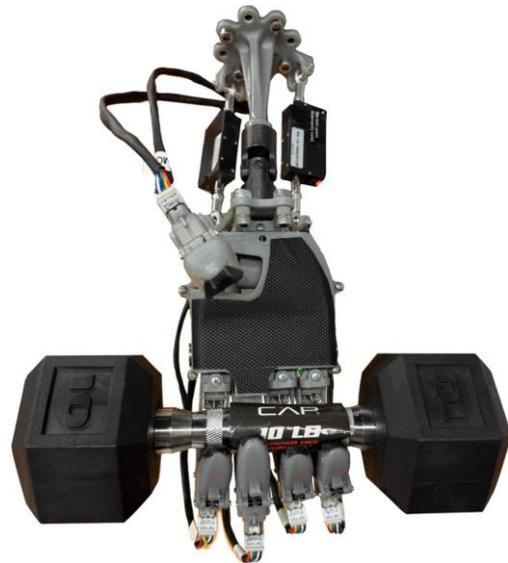
Fig. 11. Krysalis Hand passively holding a 10 lbs (4.54 kgs.) dumbbell.
