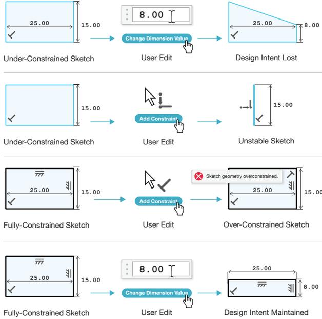
Figure 3. Comparing different outcomes when a designer updates a sketch parameter on the constrained sketch. **First row:** an under-constrained sketch only preserves a subset of the geometric relationships. **Second row:** the sketch is unstable, adding a coincident constraint flattens the geometry of the sketch. **Third row:** the sketch is over-constrained, causing the sketch to be uneditable. **Fourth row:** all geometric relationships are maintained after the parameter is updated.
