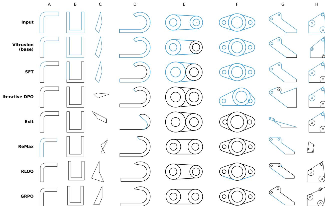
Figure 5. Visual comparison of sketches with constraints generated using a baseline model and with different post-training approaches applied. Curves are colored black when constrained and blue when not.
