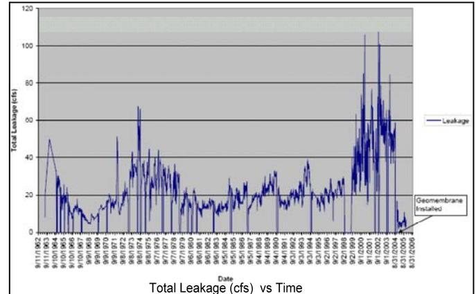
Fig. 4. – This figure from FERC's Independent Panel of Consultants Report (2006) shows a gradual upward trend in leakage rates until it was lined in 2004, dramatically reducing seepage.
