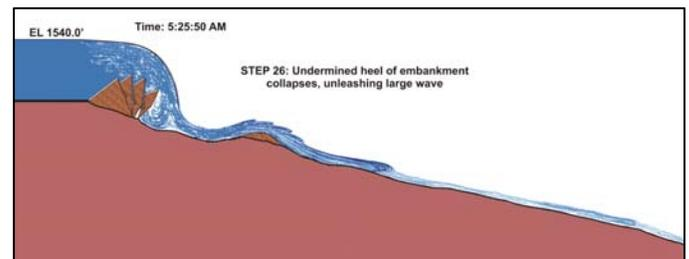
Fig. 16. – The embankment undergoes one final large collapse involving the concrete liner, sending one final surge down the slope.
